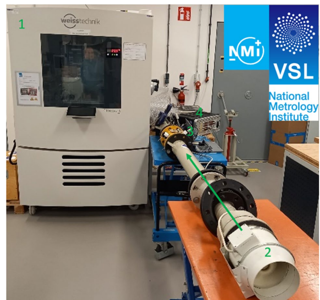
Fig. 4 Climate chamber (1), blower (2), reference flow meter (3), and its data acquisition system (4). The EFM and its control box are located within the climate chamber. The green arrow indicates the flow direction
