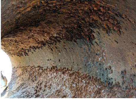
(a) Spatially non-uniform corrosion in a gas pipeline. Image: Ghorbani and Zadeh (2020), reproduced with the authors' permission.
