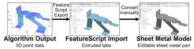
Fig. 3 CAD export pipeline: algorithm output visualized in PYVISTA (left), FEATURES import into ONSHAP (middle), and editable sheet metal model after manual conversion step (left)
