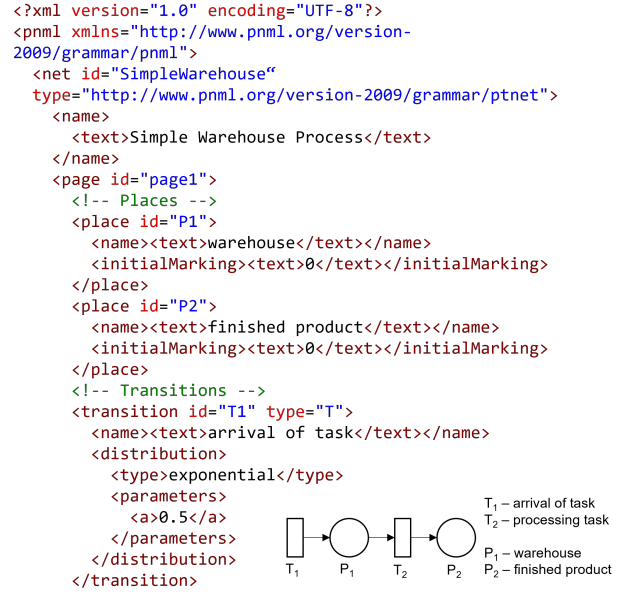
Figure 3: Graphical representation of a stochastic Petri net model and a snippet of its corresponding PNML file.
