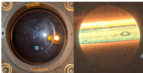
Figure 6: Radiation-damaged optical window (left) and radiation-damaged in-vacuum mirror (with synchrotron radiation present).
