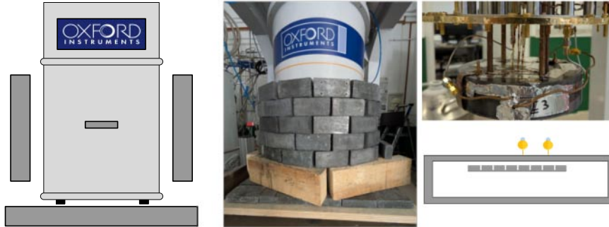
Fig. 1. – Schemes and pictures of the experimental setup consisting of a lead castle and lead pot that hosts the BULLKID detector.
