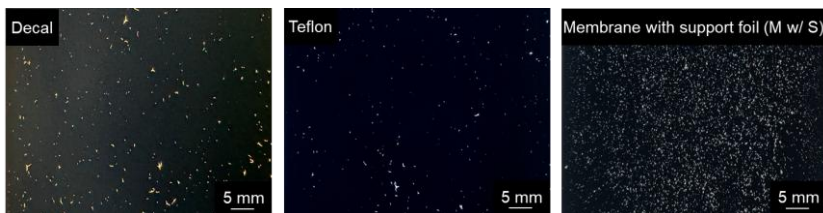
Figure 24: Influence of the substrate on the crack pattern in catalyst layers. An identical ink was applied to a decal foil, a Teflon foil and the membrane (M w/ S) and the catalyst films were dried with the same drying conditions ( T = 25\text{ }^{\circ}\text{C} , \alpha = 35\text{ W m}^{-2}\text{ K}^{-1} ). The dry film thickness is approx. 8.6 \pm 0.5\text{ }\mu\text{m} . Cracks are visible as white spots. [30]
