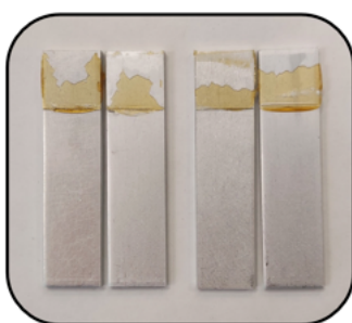
Figure 7.51 Representative adhesive-cohesive failure of lap-shear test specimens prepared with crosslinked NIPU adhesives after 1 day of RT curing.
