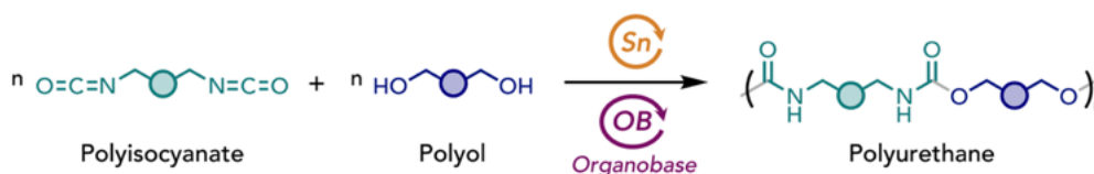
Scheme 2.1 Polyaddition reaction between polyisocyanates and polyols to form polyurethanes.
