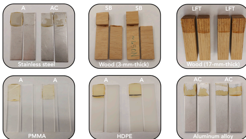
Figure 7.53 Representative failure modes (A = adhesive, AC = adhesive-cohesive, LFT = light-fiber-tear, SB = stock-break) of lap-shear test specimens prepared with NIPU adhesive formulation PJ, evaluated after 1 day of RT curing on different substrate materials.
