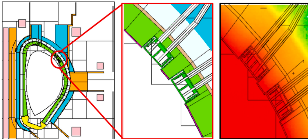
Fig. 10. Left: MCNP plot of the converted geometry with antenna. Middle: zoomed view of the converted antenna geometry, with the straps and transmission lines visible. Right: corresponding neutron-flux map in the antenna vicinity, shown on an arbitrary scale.
