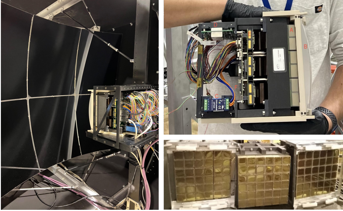
Figure 12. Photograph of the inside of the assembled EUSO-SPB2 Fluorescence Telescope (left), the three PDMs in the laboratory without the lens assembly installed (bottom right), and one PDM with lens assembly installed held by a graduate student to show the scale (top right).
