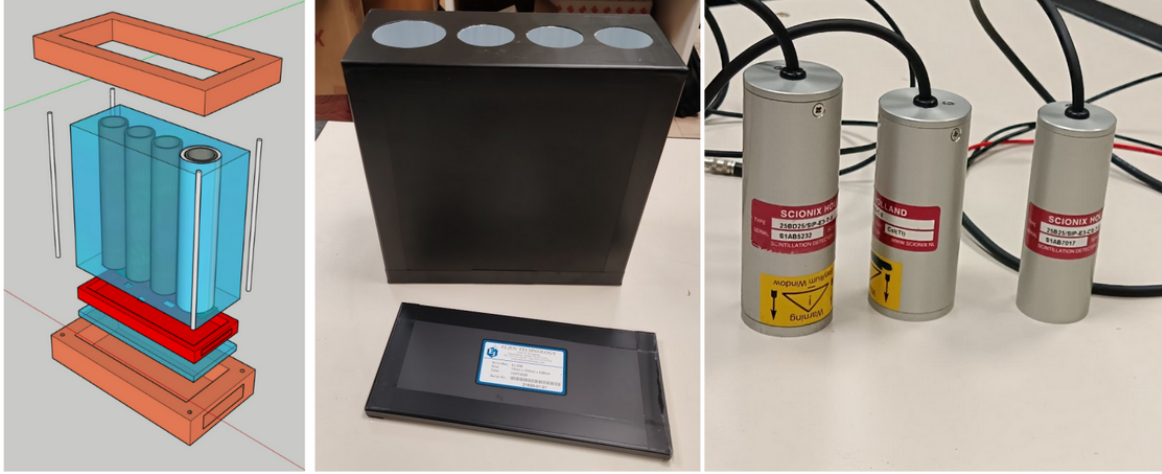
Figure 15. Left: CAD model of the X- \gamma detector ( 28 \times 16 \times 30 \text{ cm}^3 ). Cyan: anti-coincidence panels; orange: aluminum parts; red: PVC bases for lead collimators. Rightmost cylinder is the low-energy X channel (not covered by anti-coincidence to avoid absorbing low-energy X-rays). Aluminum enclosure omitted. Center: bottom view of the anti-coincidence assembly showing four collimator apertures; the smaller scintillator plate covers the openings. Right: three Scionix detectors used in the X- \gamma detector.
