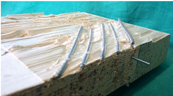
Figure 14: Plastic deformation of screws 8x300 mm.
