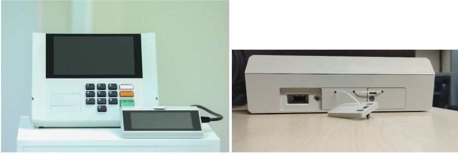
Fig. 1. (a) Brazilian voting machine, comprising the voter terminal and the poll-worker terminal. (b) Currently disabled USB port in poll-worker terminal for potential expansion.
