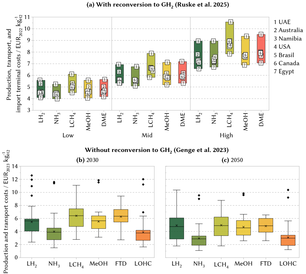
Figure 2.4: (a) Production, transport, and import terminal costs for importing liquid hydrogen ( \text{LH}_2 ), ammonia ( \text{NH}_3 ), synthetic liquid methane ( \text{LCH}_4 ), methanol ( \text{MeOH} ), and dimethyl ether ( \text{DME} ) from selected countries—such as United Arab Emirates (UAE) and United States (USA)—to Germany, including reconversion to gaseous hydrogen ( \text{GH}_2 ), shown for low, medium, and high cost scenarios. (b) 2030 and (c) 2050: Production and transport costs for importing \text{LH}_2 , \text{NH}_3 , \text{LCH}_4 , \text{MeOH} , Fischer-Tropsch diesel (FTD), and liquid organic hydrogen carriers (LOHC) to Europe from 30 different studies. The costs exclude reconversion to \text{GH}_2 . Own depiction based on data from [84, 85]; reproduced by permission.
