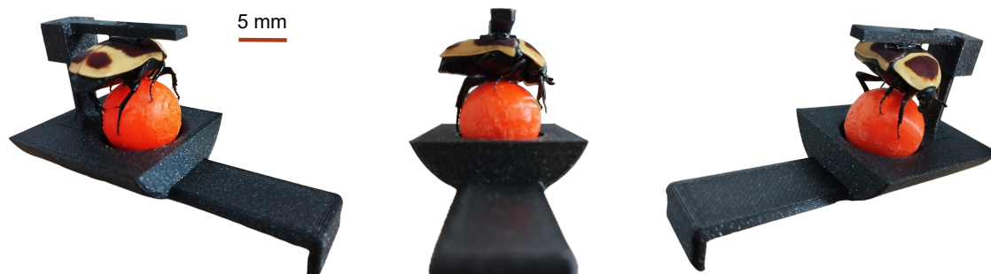
Figure 3.9: Tethered sun beetle on a spherical treadmill.
