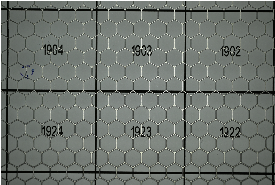
Figure 4.4: An example of one of the 336 base images taken of the cathode mesh to ease the inspection.
