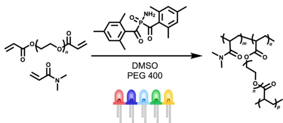
Fig. 2 Light-induced polymer network formation of the photoresin based on DMA, PEG DA 700, DMSO, PEG 400 and BAPO-NH 2 as photoinitiator.
