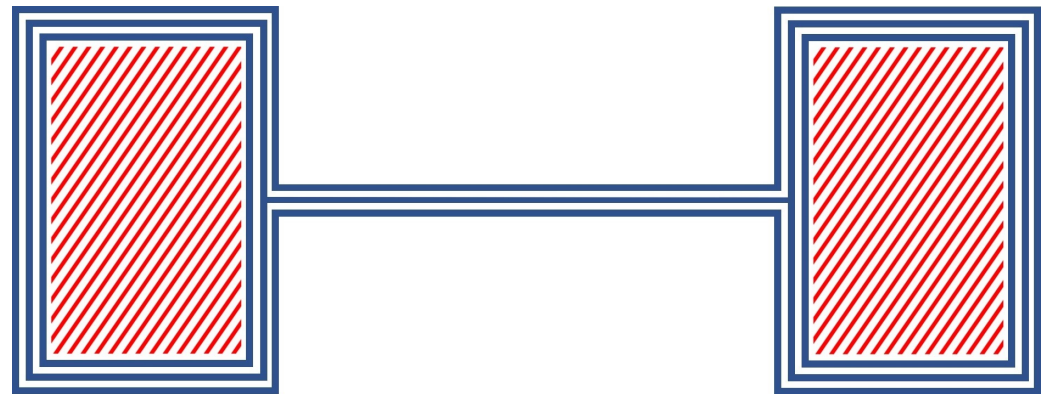
Figure 3. Schematic illustration of the scan strategy. Blue: Contour-laser-paths. Red: Hatch-paths.
