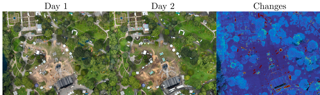
Fig. 9. Changes within the scene. On the left and center are two LiDAR scans from Day 1 and Day 2 displayed. On the right side, the changes are color coded. Red highlights major changes, while blue symbolizes no significant changes.
