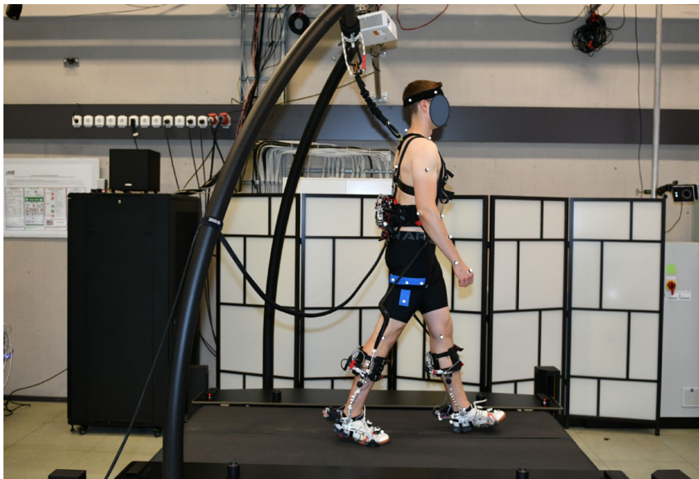
Fig. 1 Experimental setup showing a participant on the split-belt treadmill wearing the ankle exoskeleton and reflective motion-capture markers
