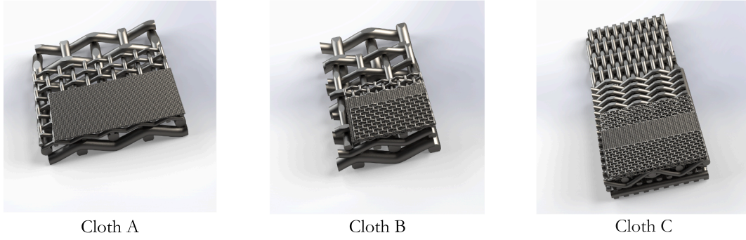
Fig. 1. Schematic structure of the composite-cloths used. The composite-cloths consist of different stacked layers that are sintered together.
