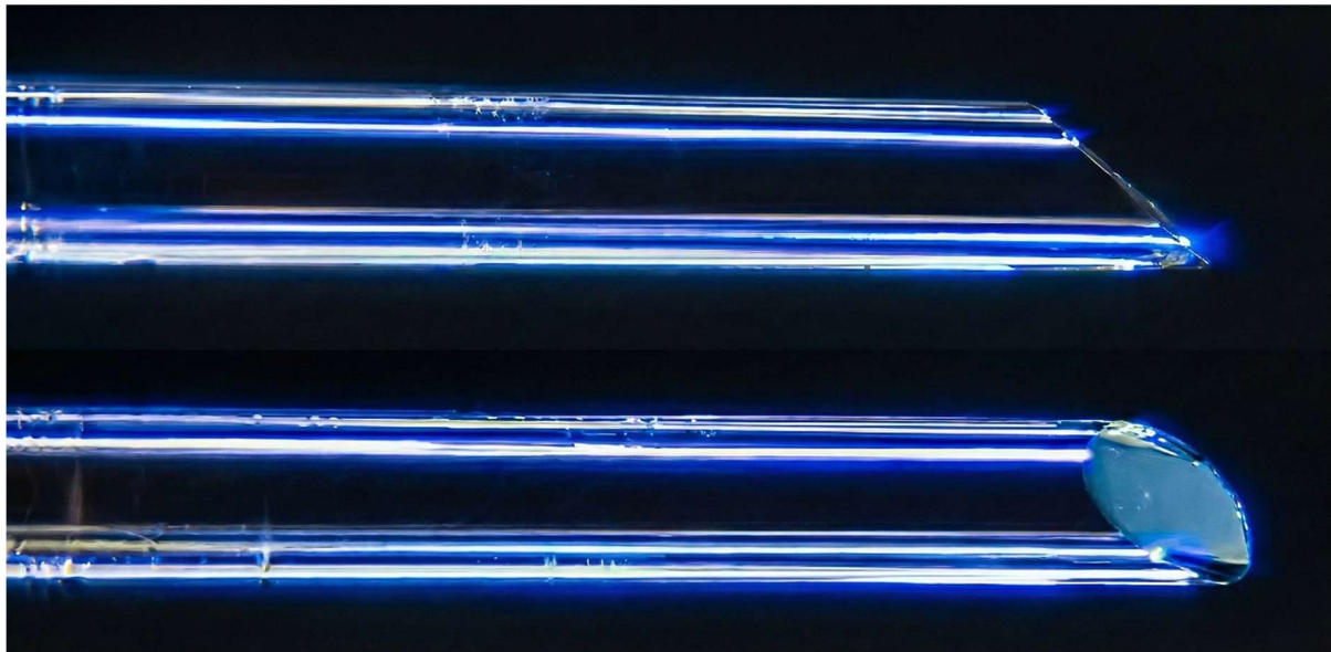
Figure 4.12: Side and top-side view of an angle-polished glass fiber (adapted from [42]).
