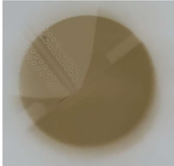
Figure 5.11: Radiation-induced discoloration of a microscope slide of a disassembled ring modulator sample due to color centers.
