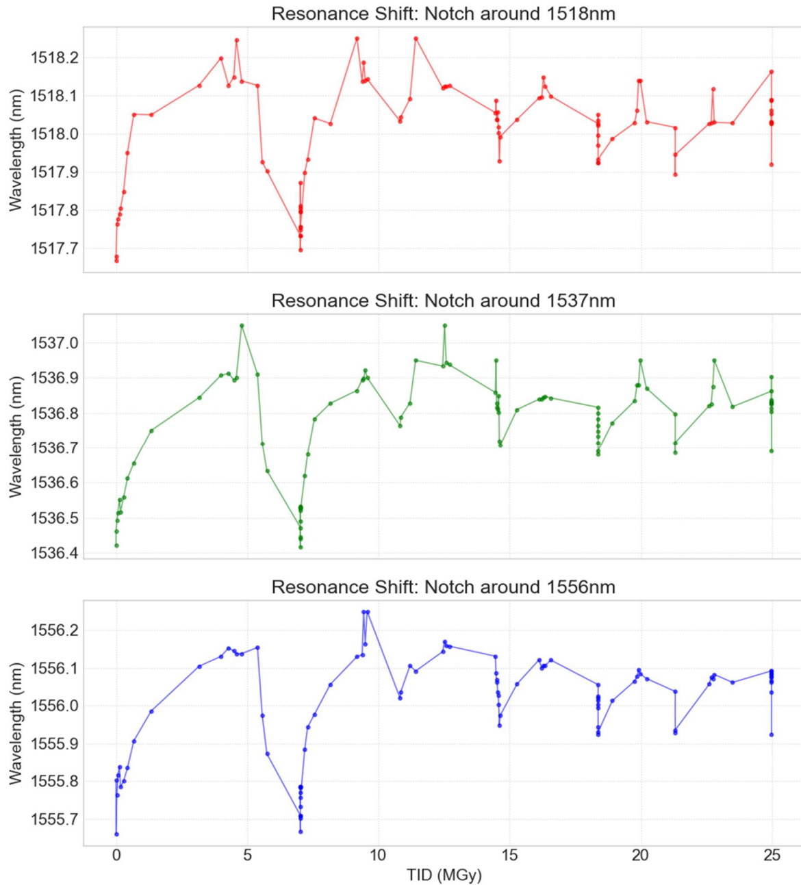
Figure 5.25: Resulting plots of the notch tracking of the DC spectra of the ring modulator sample.
