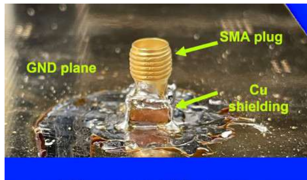
Figure 3.5: Capacitive probe implementation on the back side of the PCB (del Barrio Montañés et al. (2025)).
