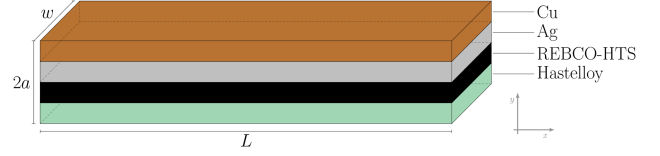
Fig. 3. Schematic sketch of the 2G-HTS tape, its layers, and the main dimensions.
