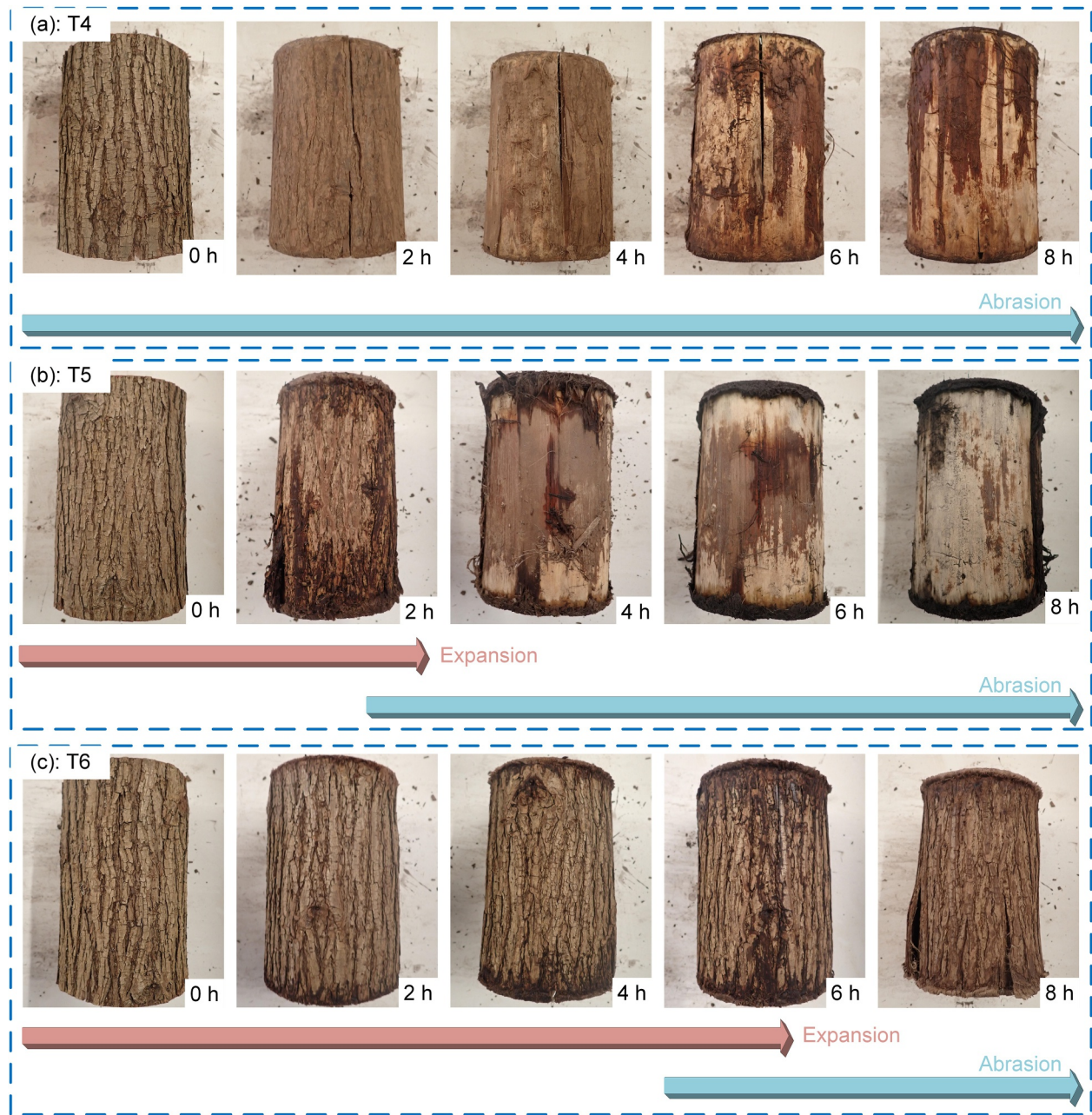
Figure 6. Debarking modes under varying flow velocities for the same water content (take sample 3 in tests T4, T5, and T6 as examples): (a) T4; (b) T5; and (c) T6.
