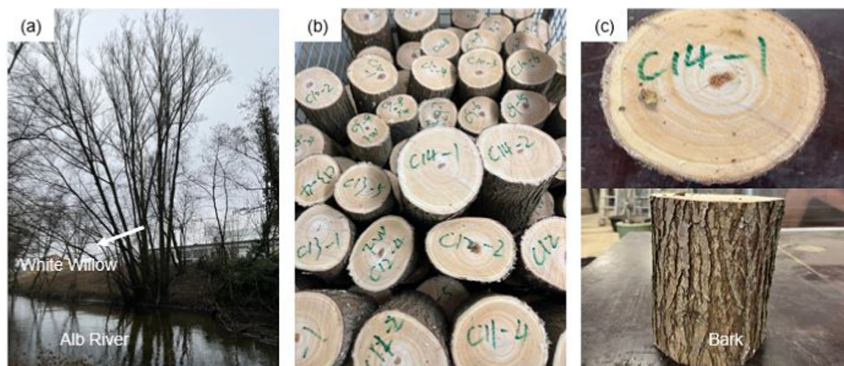
Figure 2. The trees and wood samples for experiment: (a) white willow alongside the Alb River in Karlsruhe; (b) wood samples; and (c) the size and bark of the wood samples.
