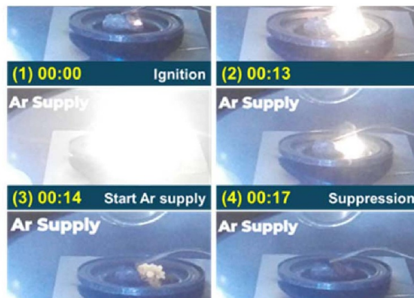
Figure 14. Experiment of lithium ignition and extinguishing by Argon gas. Reprinted from [24], Copyright (2026), with permission from Elsevier.
