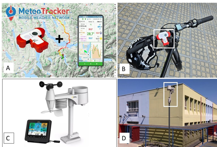
Fig. 3 The sensors used in the CityCLIM citizen science activities. A) MeteoTracker mobile weather network sensor developed by IoTopon (source: www.meteotracker.com ). B) The MeteoTracker is used by citizen scientists to collect temperature data while cycling, as shown on a participant's bicycle in Karlsruhe (outlined in white box). C) National Geographic 7-in-1 Weather Station with WIFI connectability developed by Bresser (source: www.bresser.com ). D) The National Geographic 7-in-1 Weather Station is shown here mounted on a pole beside the building of a participating school in Thessaloniki (outlined in white box)
