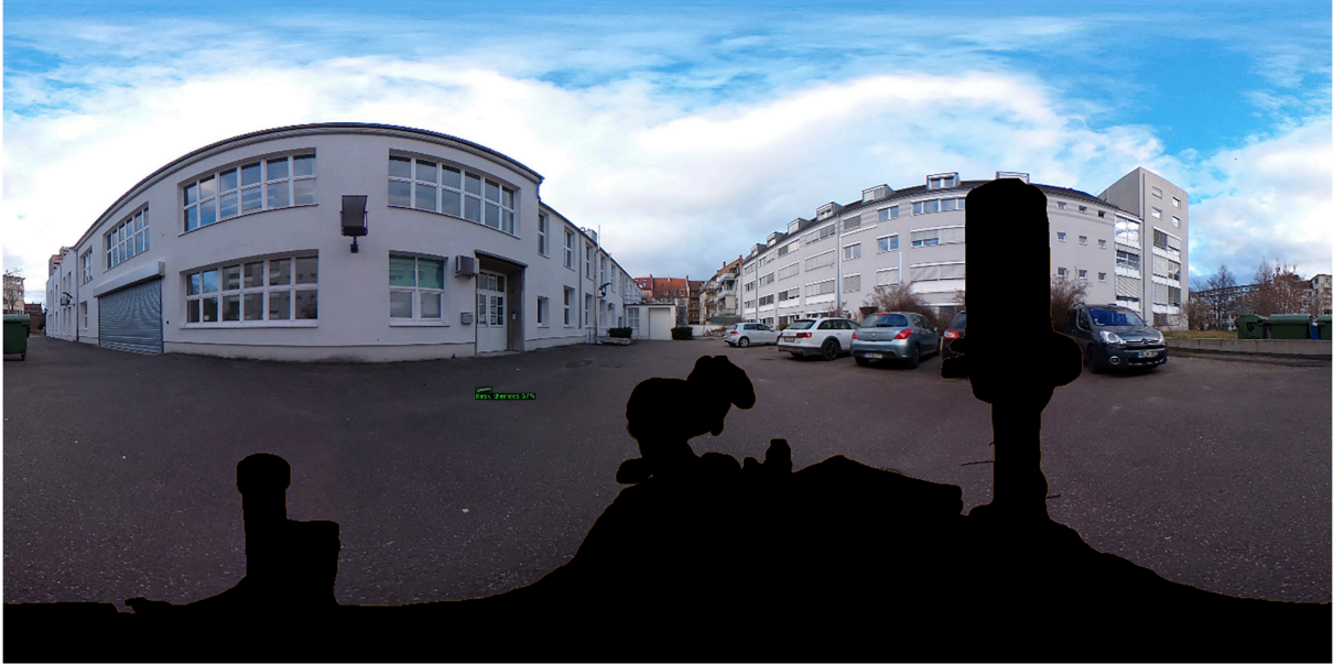
Figure 6.19: Qualitative example of the detection of a hazardous container on a wide-angle camera of the mobile robot Husky . Although the environment is cluttered and contains many metal, cylindrical objects there are no false positives. Image taken from [P8], licensed under CC BY 4.0.
