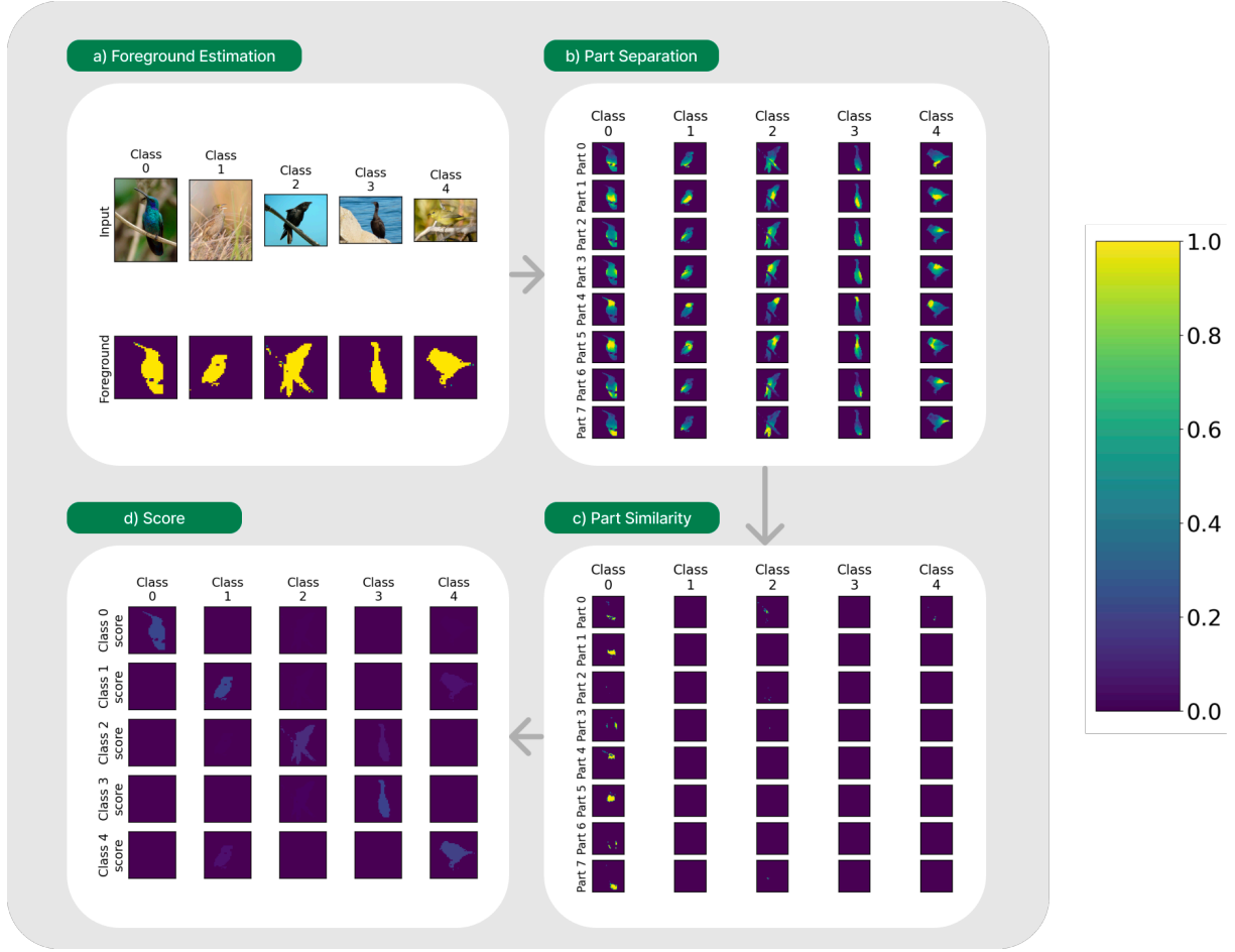
Figure 6.8: Visualization of the inference pipeline of the proposed fine-grained object recognition architecture. The shown task is a 5-way-5-shot task from the CUB-200-2011 dataset [26]. In (a) the foreground is segmented, in (b) the semantic parts are separated, in (c) the part similarity with the trained classes is estimated (note the figure only shows the similarities for the first query image input 0), and (d) presents the final class score maps. On the diagonal of (d) the birds are clearly visible, demonstrating that the similarities with the correct class are the highest and that the architecture also coarsely localizes the objects within the query image. Copyright ©2024, IEEE [P3].
