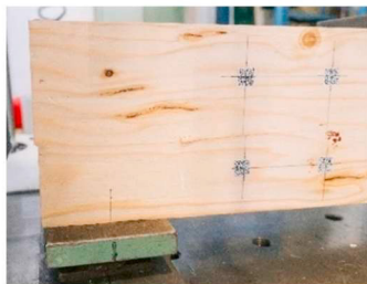
a) Shear failure of a timber ref. specimen
