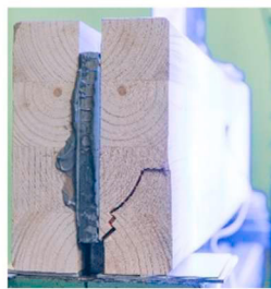
b) Shear failure of a PMPF specimen
