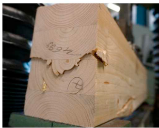
a) Shear failure of a timber reference specimen
