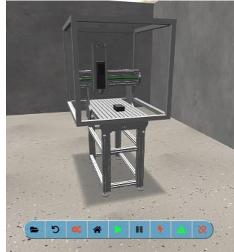
Fig. 3. Virtual twin of 3-Axis CNC machine
