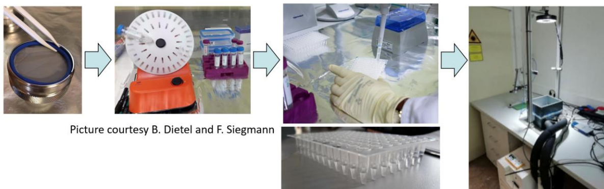
Figure 9: Offline analysis procedure with INSEKT; from left to right: The filter is taken out of the filter holder (left), placed in a tube containing Nanopure water and mounted in a rotator (center left), and the resulting suspension is pipetted into wells of a PCR plate (center right), which is then placed into the cooled aluminum box connected to a cryostat (right).
