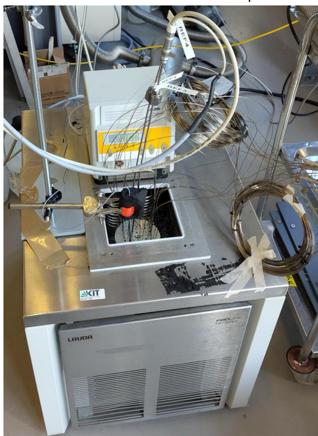
Figure 10: Example setup for calibration of droplet freezing assay temperature sensors (left) with detailed view of metal block with temperature sensors inside an ethanol bath (above).
