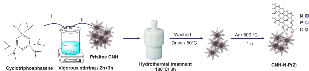
SCHEME 2 | Schematics of the single-step functionalization of CNH using molecular Hexa(N, N-dimethylamine)cyclotriphosphazene as a single-source precursor. For details, see Experimental Section (Supporting Information).
