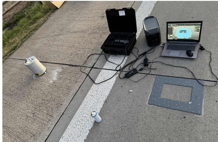
Figure A2. Setup for the 3D scan of A6_L1_M2. Power station and laptop (finalizing the scan); the scanner is in its carrying case, which includes an integrated calibration plate. The reference frame was positioned parallel to the edge of the concrete slab so that the orientation matches the direction of travel (arrow points in the x direction). On the left, you can see the ELAtexture device during a texture depth measurement on A6_L1_M1_R. The white residue comes from the vanishing scanning spray.
