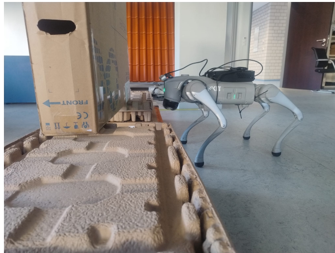
Figure 6.8: Geometric setup for the crawling task. The robot is 45 cm tall with the payload, while the cardboard obstacle provides only 27 cm clearance, so a substantial posture change is required to pass underneath.
