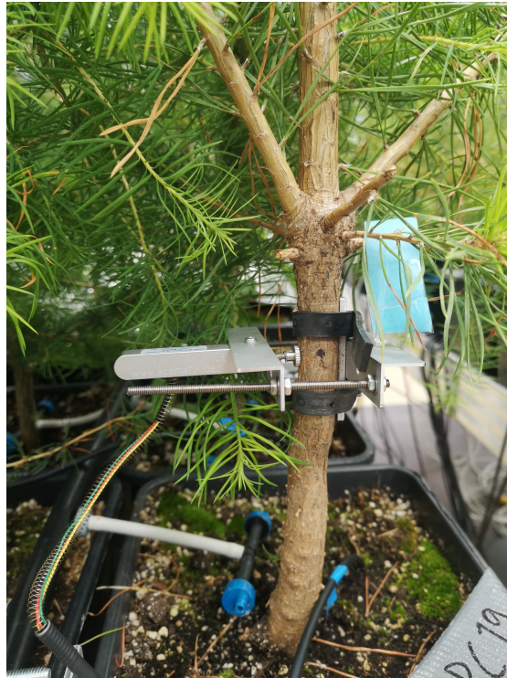
Figure S2.9: Exemplary dendrometer setup.
