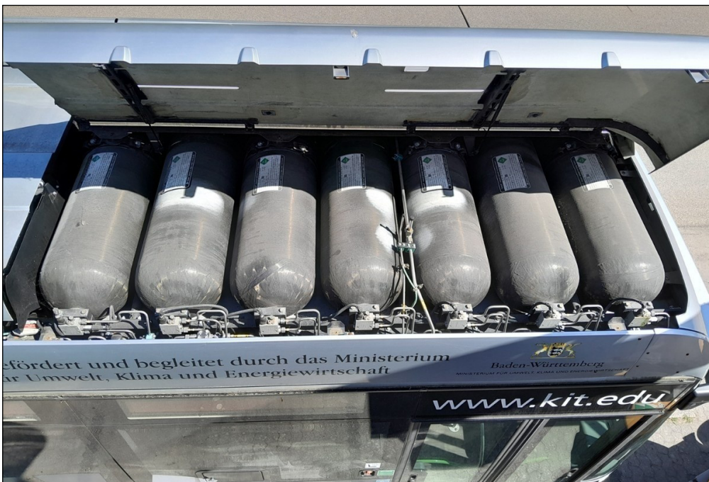
Figure 2 The seven Type III hydrogen storage tanks in the roof of a H 2 shuttle bus.
