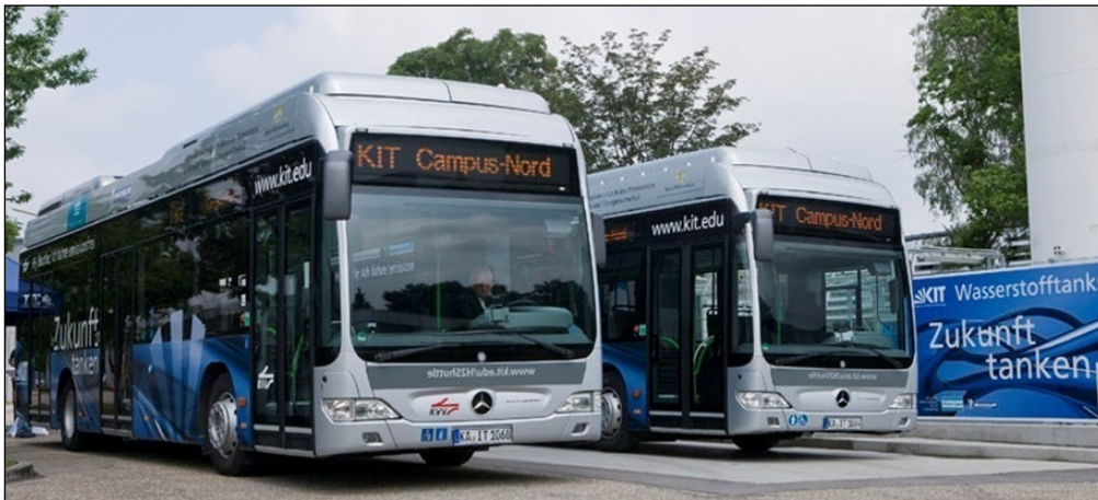
Figure 1 The two H 2 fuel cell hybrid buses of the KIT shuttle in front of the H 2 refueling station at KIT.
