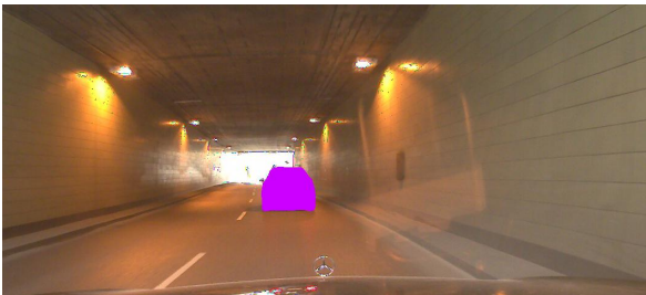
(c) Camera image of a frame in sequence 2, time t = 107.5 s [Sch+21b]. Radar motion estimation fails due to the challenging operating conditions for the radars in the tunnel.
