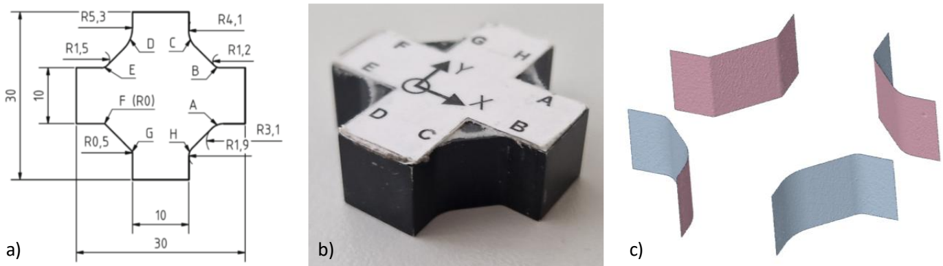
Figure 8: IIW round-robin part A notch specimen, a) dimensions, b) matt surface conditions, c) cut scan data for evaluation [23]
