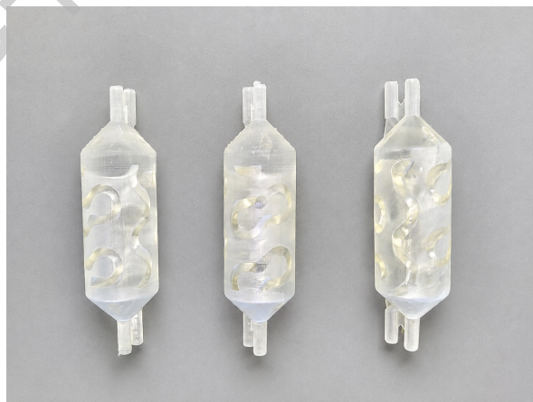
Figure 2: SLA-printed HT resin column prototypes with gyroid-type internal features used for methanol-water distillation experiment.
