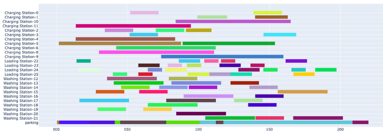
Fig. 4 Gantt diagram of a schedule based on the random heuristic
