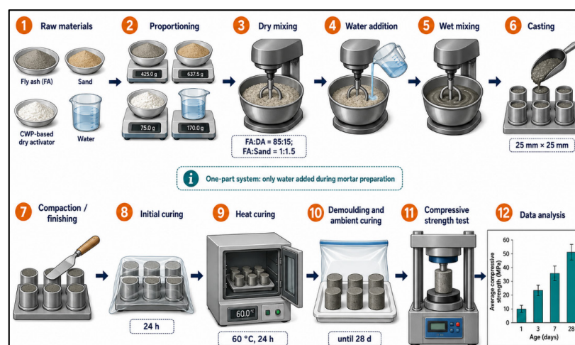
Figure 4. Methodology of one-part geopolymer mortar preparation.
