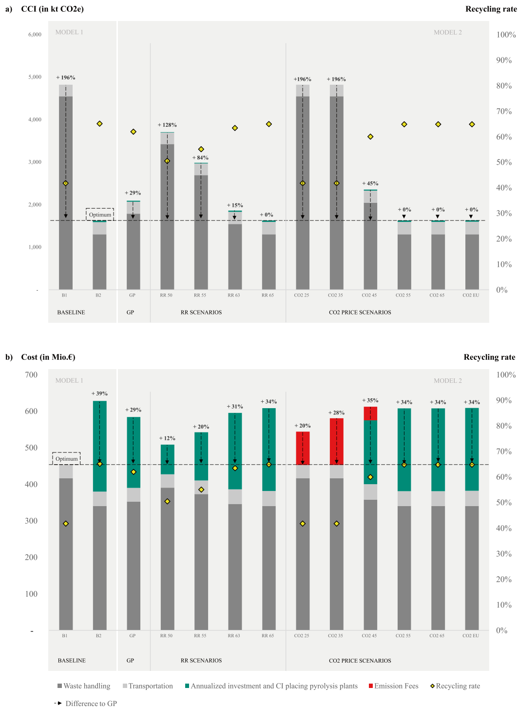
Fig. 2 Impact of different scenarios on a CO 2 e emissions (in kt CO 2 e), b costs (in Mio. €), and recycling rate (in %). All results are displayed in tabular form in Supporting Information S2.2
