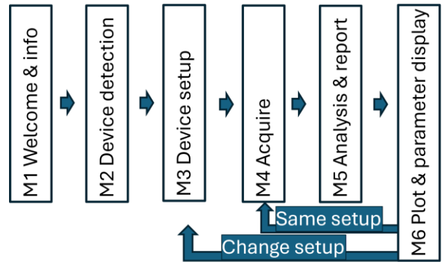
Figure 2 FiLiPulse workflow. After module M6, the operator can either continue with the same setup (M4) or change the setup (M3). Program exits are not shown in the workflow for clarity.
