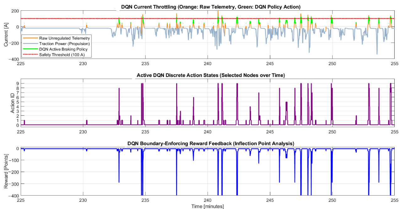
Figure 12. DQN control actions and reward (points) versus the inputs shown in Figure 11 (the vehicle speed, current I , and I_{\text{stress}} ) under the ambient temperature of 35 °C.
