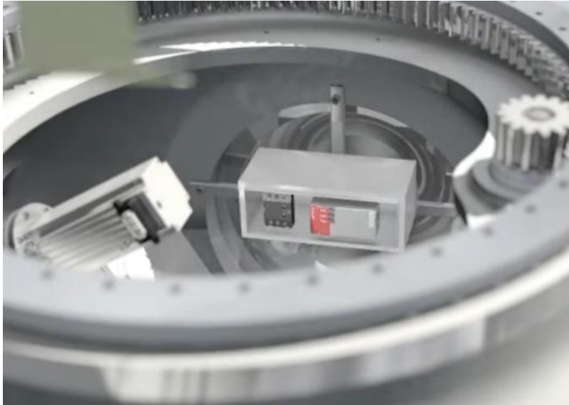
Central pitch control in hub
