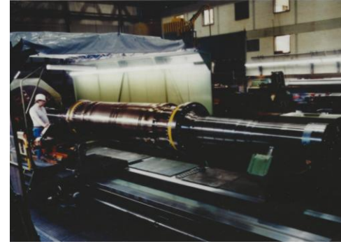
1991: Germany (Siemens) Rotor of 400 MVA NbTi experimental generator
