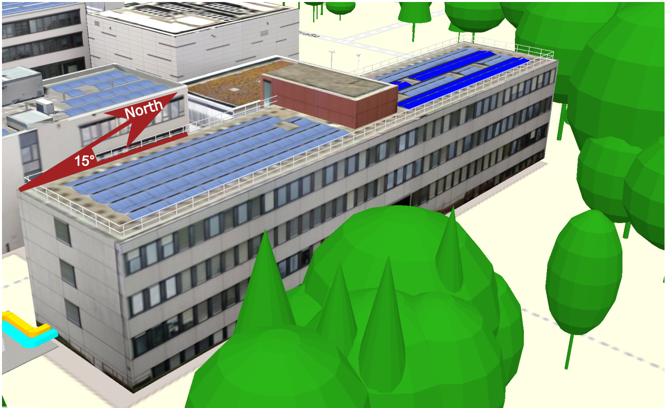
Figure 3.1: Virtual building model with investigated rooftop PV system shows the orientation of both the building axes and inclination of modules. Picture taken from the 3D campus model of the KIT/IAI [69]. Special thanks to Karl-Heinz Haeefe for extracting this schematic.
