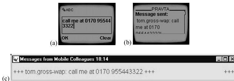
Figure 5. The PRAVTA prototype user interface: (a) send message dialogue; (b) feedback; (c) resulting tickertape on the PCs of the colleagues in the offices.
