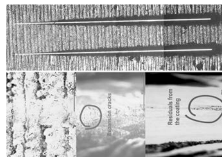
Figure 2. Micrograph of scratch trace: top: 50× magnification; bottom: 500× magnification – at the beginning, middle and end of test (from left to right).
