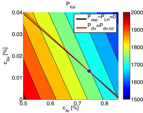
**Figure 5.** Investigation of the optimum impurity mix of Ar and Xe. Contour levels illustrate fusion power. The red and black lines show the limits of satisfying criterion (a) and (b). The blue circle marks the identified optimum impurity mix.
