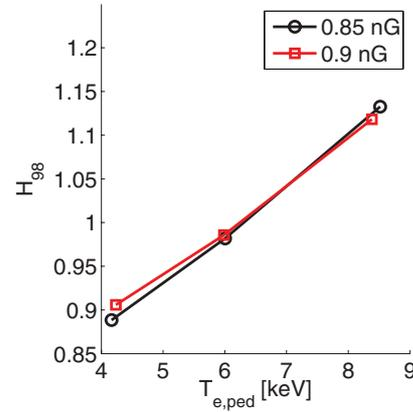
**Figure 1.** Dependence of radiation corrected confinement factor (the power injected to the H98 scaling is  $P_{heat,tot} - P_{rad,core}$ ) on the electron temperature at the pedestal top from calculations with the core transport module TGLF [6]. The electron density at the pedestal top has been set to 85 and 90% of the Greenwald density respectively.
