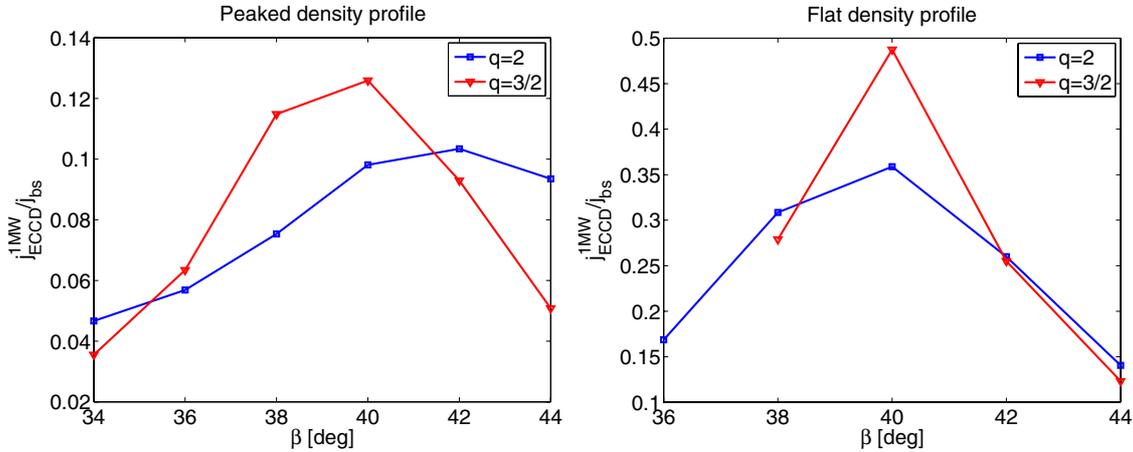
**Figure 4.** Ratio between ECCD current density and bootstrap current density at the position of the  $q = 3/2$  and  $q = 2$  surfaces, assuming 1MW injection, for flat and peaked density profiles as a function of toroidal injection angle  $\beta$ .
