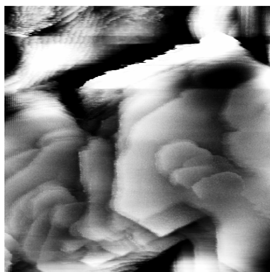
Fig. 4.10 OPD of Zn. E=-200 mV, 5 nm Image size 87×87 nm, scan rate is 3.39 Hz, I_{\text{tun}}=1 nA, E_{\text{tip}}=0 mV 0 nm
