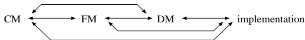
Figure 2. Different transition paths between a conceptual model and an implementation. CM = conceptual model, FM = formal model and DM = design model.
